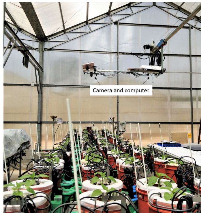
Figure 2. A view of the experimental table and the hyperspectral camera traveling above. Each plant was placed in a custom weighing lysimeter connected to Plantarray 3.0 system. Four drippers irrigated each plant while the water evaporation was restricted using a plastic cap.
